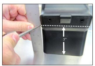
**7.** Set the factory air scoop on a workbench and mark all four corners at the three inch mark using a scratch awl. Using a straight edge and the awl, scribe a line connecting all four corners.
