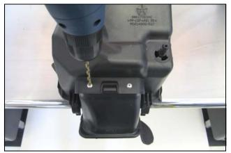
**6.** Drill out the rivet heads on the factory airbox and remove the air scoop.
