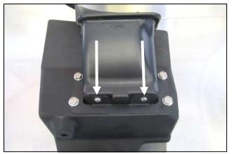
**9.** Insert the factory air scoop into the Cold Air Box and secure it using two  $8-32 \times 3/8$ " Button Head Bolts , #8 Flat Washers, and #8 Kep Nuts.
