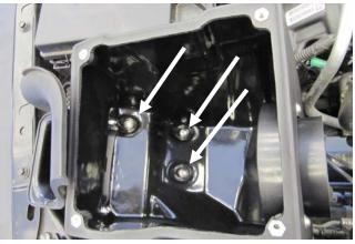
**11.** Mount the Cold Air Box assembly in the inner fender using the three 3/8" x 1 1/2" Button Head Bolts.
