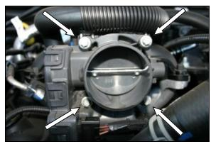
2. Using a 6 point 5/16" socket, remove the 4 bolts that hold the throttle body to the intake manifold.
