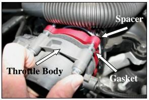
3. Install the Poweraid Spacer and the fiber gasket between the intake manifold, and the throttle body, as shown. Tighten all 4 throttle body bolts evenly, to the manufacturer's specifications. **Do Not Over Tighten The Bolts!** \*Note: Poweraid spacer must be installed with bore protruding into intake manifold away from throttle body. Incorrect installation will hinder performance. Reference picture below for spacer orientation.
