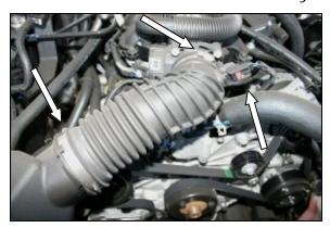
1. <u>Disconnect the negative battery cable!</u> Loosen 2 hose clamps on each end of the factory intake tube. Slide the red locking tab, and then squeeze the black tab, and disconnect the intake tube temperature sensor wiring harness. Remove the tube from the vehicle.
