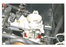
**5.** Install one gasket (#4) on the intake manifold, then the Poweraid spacer (#1), with the other gasket (#4) on top of it. Next install the throttle body using the four provided 6mmx50mm bolts (#2) and washers (#3), and tighten to manufacture's specifications.
