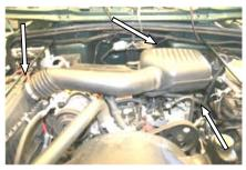
**7.** Re-connect the intake tube to the airbox, reconnect the breather hose, and tighten all hose clamps.
