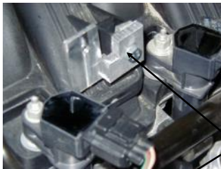
Ref. "C" (2) Air Box Ext. Plates (2) 6mmx20mm Hex Bolts (2) 6mm Flat Washers
