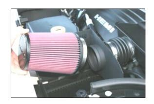
**8.** <u>Install the Airaid Premium Filter</u> (#1) onto the tube on the Quick Fit Panels, and tighten the clamp.
