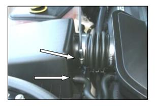
**1. Disconnect the negative battery cable.** Using a 5/16" socket, loosen the hose clamp on the factory airbox lid. Twist and remove the breather hose from the factory airbox lid.
