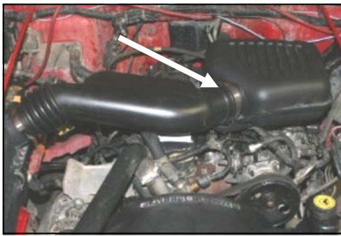
1. Disconnect the negative battery cable. Loosen the hose clamp that holds the factory intake tube to the resonator.
