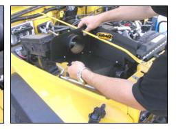
12. Carefully slide the Airaid Cool Air Dam assembly over the passenger side radiator support rod. Be careful not to scratch the paint. Insert the rubber grommet into the panel for final positioning of the assembly.
