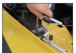
**5.** Using a 5/16" socket, remove the three nuts and bolts mounting the factory air filter housing to inner fender. Remove air filter housing.
