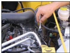
2. Loosen hose clamps on both ends of factory intake tube. Remove intake tube from engine.
