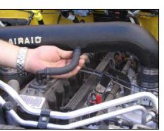
**26.** Connect the other end of the valve cover hose to the intake tube. Secure both ends of the hose using the supplied black speed clamps.
