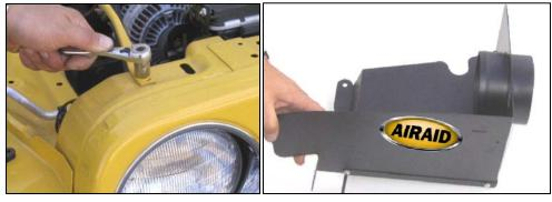
9. Using a 13mm socket, remove the radiator rod support bolt on the passenger side. Retain bolt for later use.
