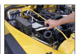
4. Remove factory air filter from airbox.
