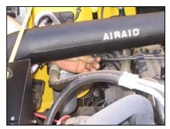
**23.** Mount the Airaid intake tube to the valve cover bracket using the supplied <sup>1</sup>/4" bolt and washer as shown above.
