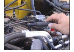
**19.** Install the supplied rubber hose on the factory plastic valve cover breather fitting.
