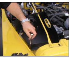
**14.** Using the supplied  $\frac{1}{4} \ge 20$  nut, bolt and washers, mount the front of the Airaid Cool Air Dam to the inner fender.
