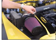
**27.** Install the Airaid Premium Filter on the Cool Air Dam assembly. Secure the filter using the supplied hose clamp.
