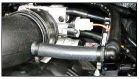
15. 2002-03 Models: Install one end of the provided  $90^{\circ}$  barbed fitting (#22) into the factory breather hose and then connect the supplied 1/2" breather hose (#21) to the other end. Connect the hose to the nipple on the Airaid intake tube. Secure all three connections with the provided #16 Speed Clamps (#17).
