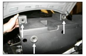
**8.** Install the factory grommets removed in step #3 into the bottom of the **CAB** at the locations shown here.
