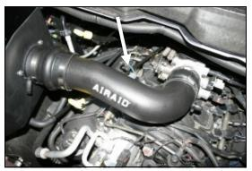
13. Slide the Airaid intake tube into the hump hose first, and then onto the throttle body. Adjust for fit, and then tighten the two remaining hose clamps. 2003-12 Models: Reconnect the temperature sensor wiring harness to the sensor in the tube. (It may be necessary to remove the tape on the wiring harness, pull out enough wire to reach the temperature sensor, and then retape the harness ).
