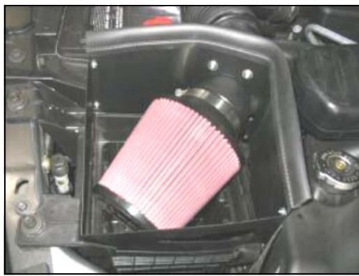
17. Install the Airaid Premium Filter (#1) onto the end of the air filter adapter. Install the weather strip (#9) onto the top of the Airaid Quick Fit Panels. ( Note: start from one end and work your way around to insure proper alignment of the weather strip. )
