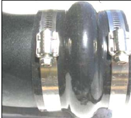
14. Install the hump hose (#7) and coupler (#8) onto the Airaid Intake Tube using four #60 hose clamps (#18). The coupler is positioned on the throttle body end and the hump hose is positioned on the air filter adapter end of the tube.
