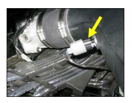
**16.** Re-connect air temperature sensor connector.
