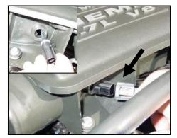
**3.** Disconnect the air temperature sensor connector on the front of the factory resonator. Next, twist the temperature sensor and remove it from the factory intake resonator. (Retain for later use with Airaid intake).
