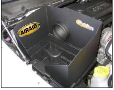
**8.** Position the Airaid Cool Air Dam in place of the original air box lid. Snap in place. Apply the Airaid Foil Decal onto the Panel as shown.
