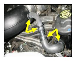
17. 2003 Models Only: Use the plastic barbed fitting and ½" hose provided; connect factory vent hose to Airaid intake tube & secure the ½" hose with (2) #16 black speed clamps provided. Secure factory vent hose with (2) #22 black speed clamps provided.
