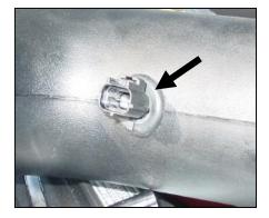
**12.** Install the rubber grommet into the hole on the back side of the Airaid tube & insert the factory air temp sensor into grommet.
