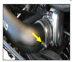
**18.** <u>2004-05 Models Only:</u> Slide the black rubber cap over the nipple near the throttle body end of the Airaid Tube.
