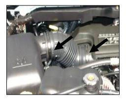
1. Disconnect the negative battery cable, and remove the factory "accordion" style intake hose by loosening the two factory clamps.
