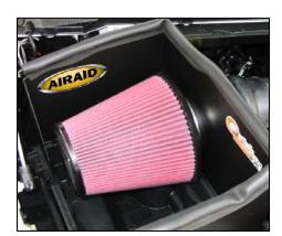
**9.** Mount the Airaid Premium filter inside the Cool Air Dam & secure with hose clamp provided.
