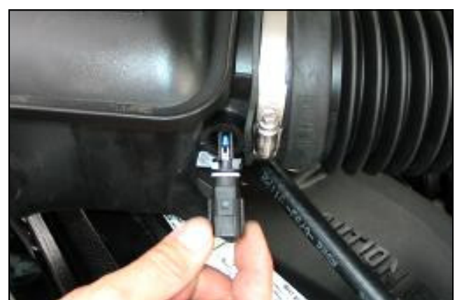
6. 2003-05 Models Only: Disconnect air temperature sensor wire on back of factory throttle body air chamber and remove sensor. Retain sensor for later use with the Airaid Intake System.
