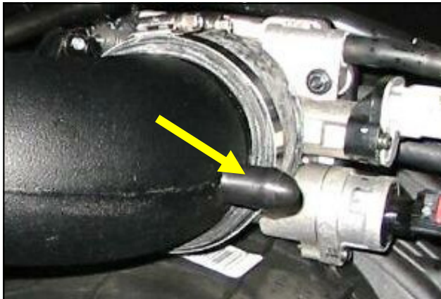
16. 2004-05 Models Only: Slide the provided rubber cap over the nipple at the throttle body end of the Airaid tube.
