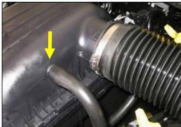
2. 2004-05 Models Only: Disconnect the factory breather hose from the factory air box lid.
