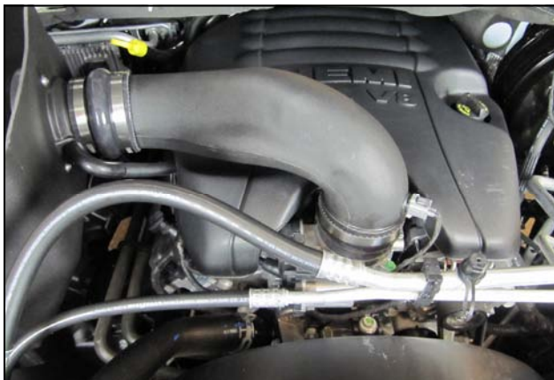
16. Install the Intake Tube, Hump Hose side first, onto the Cool Air Box, then onto the throttlebody. Align all four Clamps and tighten them. Reconnect the air temperature sensor.
