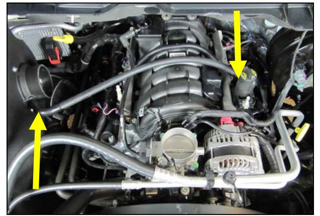
12. Install the Elbow side of the Airaid PCV line onto the Barbed Fitting on the Cool Air Box and connect the other side to the factory valve cover elbow.
