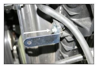
**6.** Install the L-bracket (#20) onto the radiator shroud
