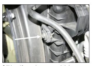
5. Using a 13mm socket remove one bolt that secures
