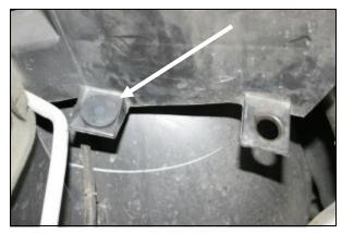
**7.** Install the supplied well nut (#16) into the factory airbox mounting hole closest to the fender as shown.
