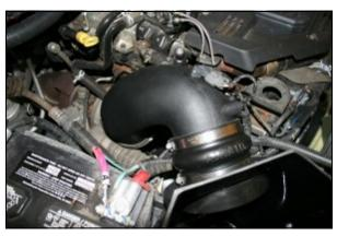
**11.** Install the Airaid Intake Tube (#2) into the factory turbo elbow and then into the hump hose. Adjust for fit, and then tighten all three hose clamps. Reinstall the intake temperature sensor and Mass Air Flow sensor into the Airaid Intake Tube using three 8-32 button head screws (#7) and #8 flat washers (#8). **Do Not Use The Factory Screws!** Reinstall the factory wiring harness anchor into the hole in the Airaid Intake Tube.
