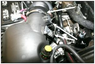
1. Disconnect the negative battery cables. A) Using the supplied #20 Torx bit, remove two screws from the Mass Air Flow sensor, and one screw from the temperature sensor. Remove both sensors and the wiring harness anchor from the airbox lid, and set them aside. B) Loosen the hose clamp that holds the factory intake tube to the airbox lid.
