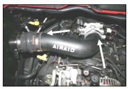
**11.** Install the Modular Intake Tube (#3) into the hump hose first and then into the factory coupler. Adjust for fit, and then tighten all 3 hose clamps.
