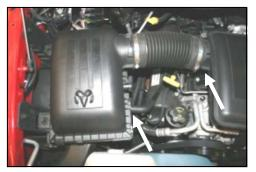
1. Disconnect the negative battery cable! Loosen the hose clamp on the resonator. Disconnect the breather hose going into the factory airbox lid.
