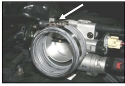
**10.** Install a #56 hose clamp (#6) on the factory throttle body coupler. Leave loose for now.
