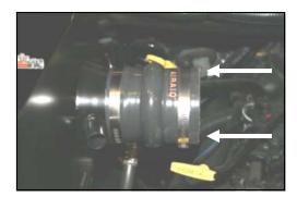
**9.** Install the urethane hump hose (#4) onto the tube on the CAD using two #60 hose clamps (#7). Leave clamps loose.
