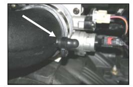
**14.** Install the provided rubber cap (#11), and speed clamp (#8) onto the nipple on the Modular Intake Tube (#3).
