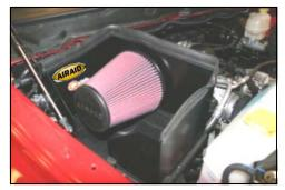
**15.** Install the Airaid Premium Filter (#1) onto the tube on the CAD and tighten the hose clamp. Next install the weather strip (#5) on the top of the CAD as shown. Apply the Airaid Foil Decal onto the Panel as shown.
