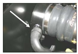
**12.** Install the provided #24 speed clamp (#9) over the factory breather hose, then slide the hose onto the nipple on the CAD. Squeeze the clamp to secure the hose.
