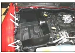
**8.** Install the Cool Air Dam (#2) onto the factory airbox base by sliding the tabs on the base thru the CAD and then adjust the sides to fit. Relatch the 4 clips to hold the CAD securely in place.
