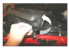
**6.** Gently twist the air temperature sensor counterclockwise and remove it from the resonator.
