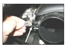
**3.** Squeeze the tab on the connector, and disconnect the air intake temperature sensor on the back of the resonator.
