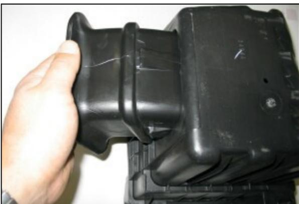
4. Using a flat blade screwdriver, carefully unsnap the box inlet from the base and remove it. Reinstall the factory base in the engine compartment with out the inlet.
