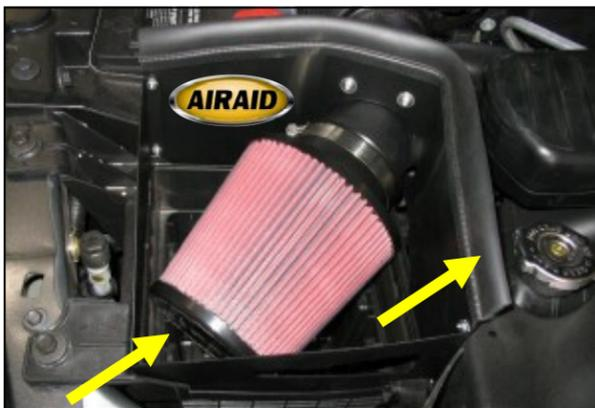
16. Install the Airaid Premium Filter on the end of the air filter adapter. Install the supplied weather strip on the Quick Fit panel. Apply the Airaid Foil Decal onto the Panel as shown.
