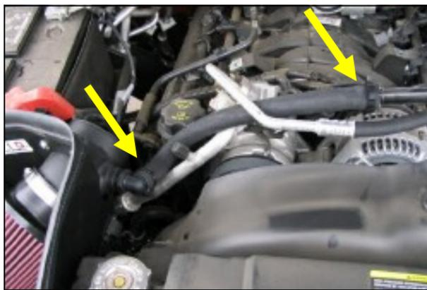
11. Using the supplied pre-formed 3/4" breather hose, connect the nylon fitting to the remaining plastic factory hose as shown. Fasten both ends of the hose using the supplied nylon speed clamps. Adjust the fitting downward to clear the factory intake tube assembly.
