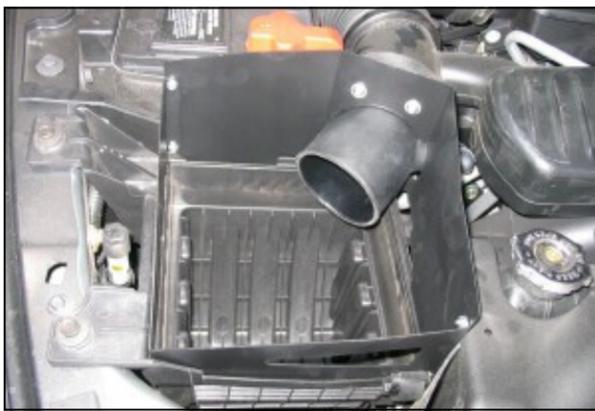
10. Install the Airaid Quick Fit assembly on top of the factory air filter base. Relatch the clips, and tighten the hose clamp.
