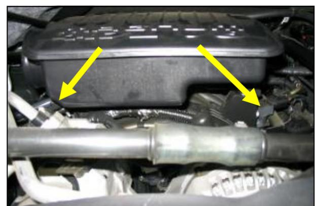
6. Loosen the two 10mm bolts mounting the factory air box to the intake manifold and remove from vehicle.
