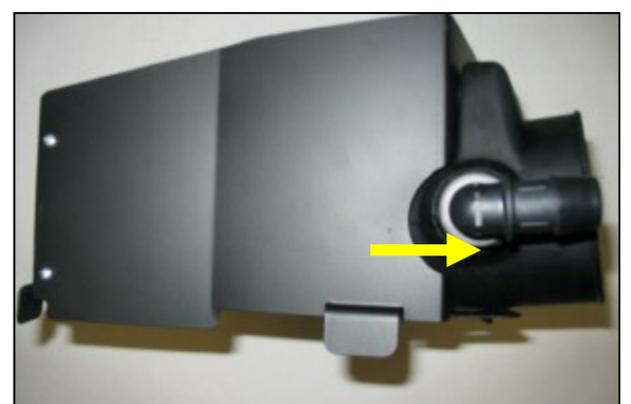
9. Install the supplied nylon fitting into the air filter adapter as shown.
