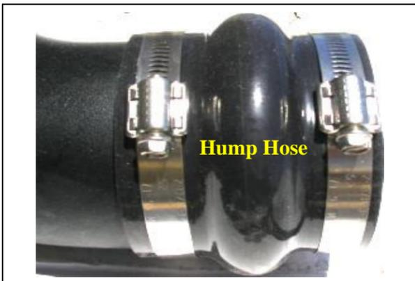
13. Slide the hump hose on to the straight end of Airaid intake tube with two #60 hose clamps. (Note: Leave hose clamps loose until final assembly).
