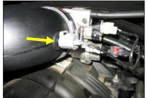
15. Install the supplied rubber grommet and factory air temperature sensor into the Airaid intake tube. Next, reconnect the factory electrical connector onto the sensor.
