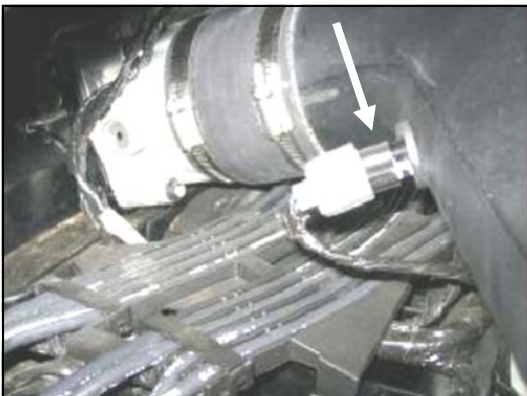
16. Reconnect the factory air temperature sensor wiring harness to the sensor.
