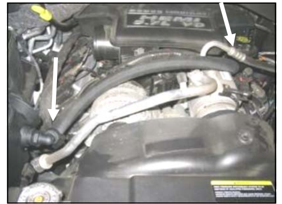
12. Remove the factory breather hose. Connect one end of the 3/4" x 25" hose (#5) to the nylon fitting and the other to the oil fill nipple as shown. Secure each end using one #24 Speed Clamp (#16). Adjust the nylon fitting downward to clear the Airaid Intake Tube assembly.
