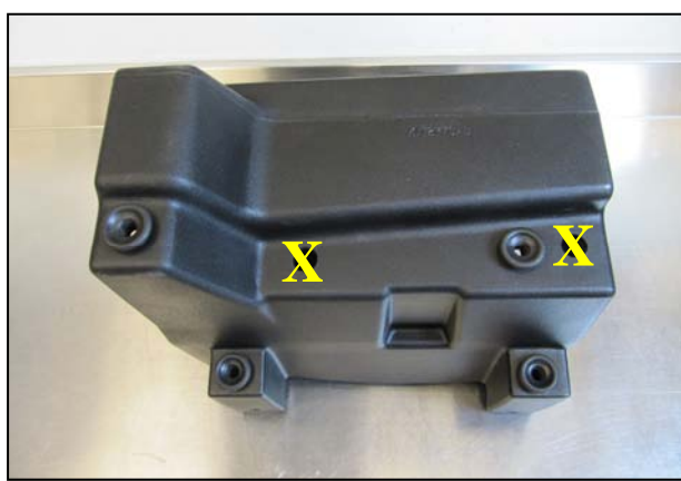
5. Transfer the 4 factory air box grommets into the Airaid Cool Air Box as shown. Note: Two of the holes do not receive grommets.
