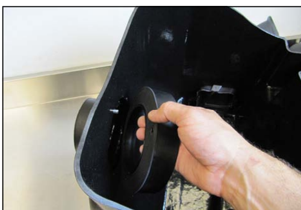
8. Mount the Filter Adapter and Gasket inside the Cool Air Box as shown using the three sets of 1/4-20 Button Head Screws (#7) and 1/4" Flat Washers (#6).
