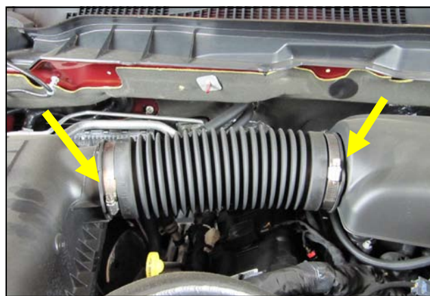
1. Disconnect The Negative Battery Terminal! Loosen one hose clamp at each end of the air intake tube and remove it from the vehicle.
