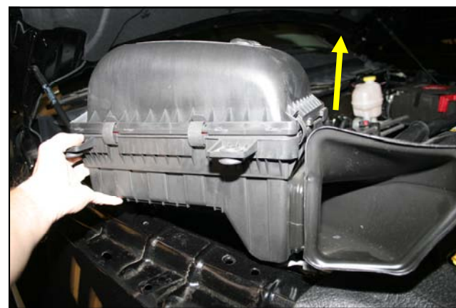
3. Rock the air box back and forth as you are lifting it straight up to remove it from the vehicle. It is only held in by grommets.
