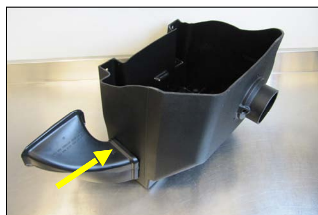
6. Transfer the scoop from the factory air box into the Airaid Cool Air Box as shown.
