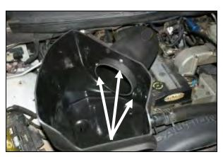
**4.** Attach the Intake Tube (#2) to the Cool Air Box, (CAB) (#3) using three 1/4" Button Head Bolts (#7) and Flat Washers (#8) as shown. Do not fully tighten the bolts at this time.
