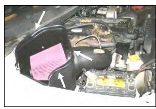
9. <u>Install the Airaid Premium Filter</u> (#1) onto the Intake tube as shown and tighten the clamp. Install the Weatherstrip (#6) onto the top edge of the **CAB** staring from the front and work your way back
