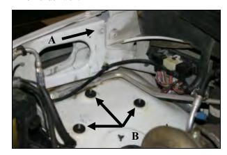
**6. A**) Remove the Factory 8mm fender bolt and set aside, it will be reused later in step **8**. **B**) Place the 1/4" I.D. Grommets (#12) over each of the three studs on the inner fender.
