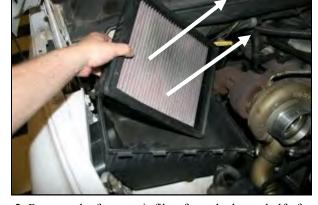
**2.** Remove the factory air filter from the lower half of the factory airbox.
