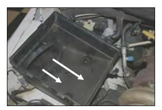
**3.** Locate the fender air scoop inside of the factory air box and remove it by pulling outward. The remaining factory airbox half can now be removed by simply pulling upward and off of the mounting studs on the inner fender well.
