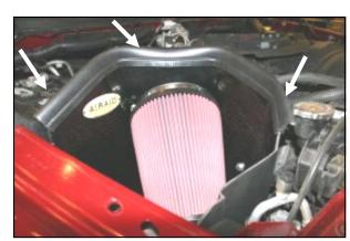
**12.** Install the Airaid Premium Filter (#1) onto the filter adapter and tighten the clamp. Install the weather strip onto the top of the **CAB** starting at the right fender and working your way towards the radiator.
