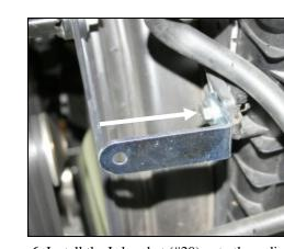
**6.** Install the L-bracket (#20) onto the radiator shroud as shown using one M8 x 30mm bolt (#14) and one flat washer (#12) as shown. Leave the bolt slightly loose for now.
