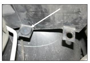
**7.** Install the supplied well nut (#16) into the factory airbox mounting hole closest to the fender as shown.
