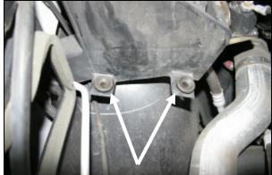
**4.** Remove the two grommets that held the factory airbox in position.
