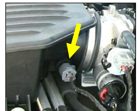
4. If your vehicle is equipped with an air temperature sensor, disconnect and remove the sensor & retain for later installation with Airaid kit.
