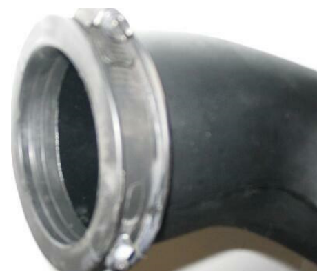
11. Reinstall factory throttle body coupler onto smaller end of intake tube.
