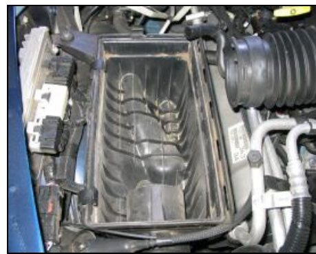
3. Unclip the factory air box lid and remove the lid and factory air filter from vehicle.
