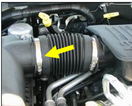
1. Disconnect negative battery cable and loosen the intake tube clamp.
