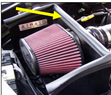
9. Press the weather seal onto the top of the Airaid Cool Air Dam. (Hint: begin at a corner and work the weather strip towards the ends)
