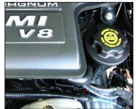
**4. 2003 Models:** Disconnect & remove the crankcase vent hose from the front of the factory resonator.
