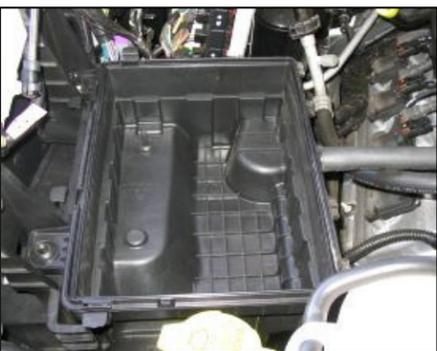
**7.** Unclip & remove the factory air box lid and factory air filter.
