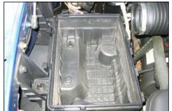
3. Unsnap and remove the factory air box lid, tube, & factory air filter.
