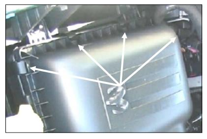
**2.** Unlatch the four factory airbox clips, and then remove the airbox lid and air filter from the factory airbox base.
