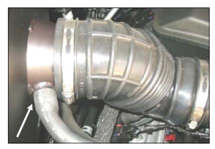
**6. 2004-2005 Models Only**: Reconnect the factory breather hose to the nipple on the **CAD** and secure it using one #24 speed clamp (#4).
