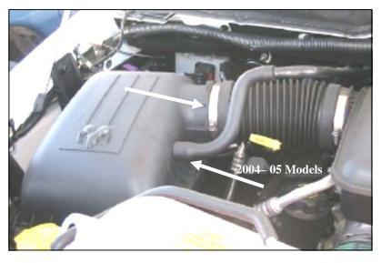
1. Disconnect the negative battery cable! Loosen the hose clamp on the factory airbox lid. **2004-05 Models Only**: Disconnect the breather hose from the factory airbox lid.
