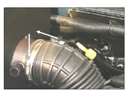
4. Reconnect the factory intake tube onto the CAD, and tighten the factory hose clamp.
