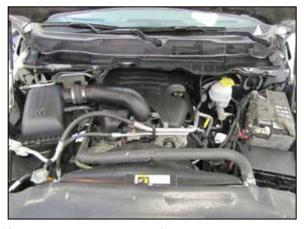
**10. Double check your work!**Make sure there is no foreign material in the intake path. Make sure all clamps, hoses, bolts, and screws are tight. Double check the hood clearance!
