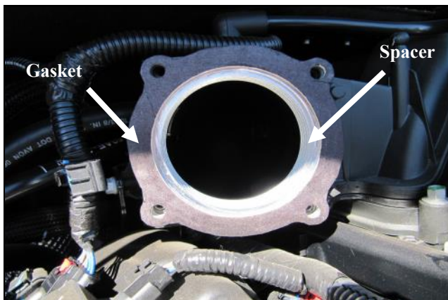
5. Insert the PowerAid spacer into the intake manifold. The gasket will go between the PowerAid and the throttlebody. *Note: Poweraid spacer must be installed with bore protruding into intake manifold away from throttle body. Incorrect installation will hinder performance. Reference picture below for spacer orientation.
