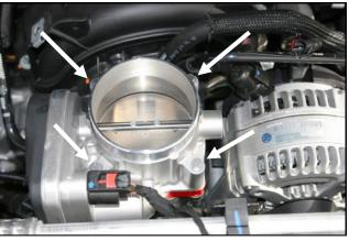
**5.** Reinstall the throttlebody on top of the Poweraid Spacer using the four bolts and the washers that were selected in step 3. Tighten the bolts evenly, in an X pattern, to the vehicle manufacturers specifications.
