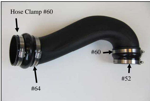
14. Slide the Coupler, Hump Hose and Clamps onto the Airaid Intake Tube as shown. Do not tighten the Clamps at this time. Refer to the line drawing and packing list for
