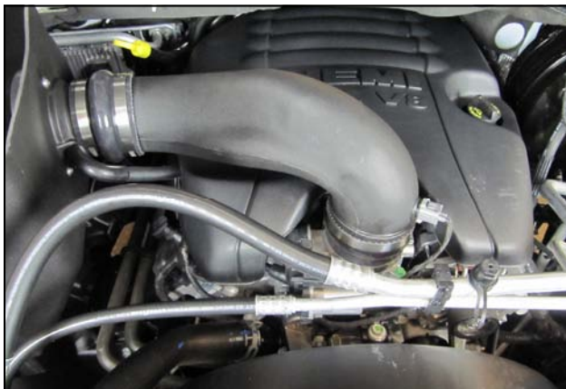
16. Install the Intake Tube, Hump Hose side first, onto the Cool Air Box, then onto the throttlebody. Align all four Clamps and tighten them. Reconnect the air temperature sensor.
