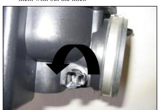
7. Turn the air temperature sensor ½ turn and remove from the air box. Retain sensor for later use.
