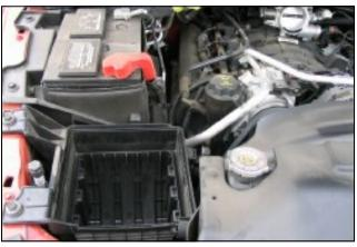
**3.** Unlatch the metal clips and remove the lid from air box base. Using a 13mm socket, remove the air box base from the engine compartment.
