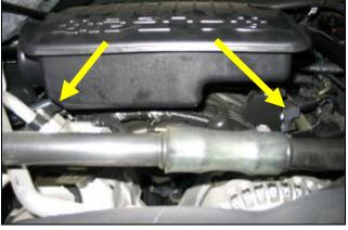
**6.** Loosen the two 10mm bolts mounting the factory air box to the intake manifold and remove from vehicle.
