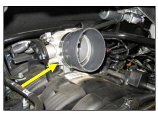
**12.** Install the supplied reducing coupler and #52 hose clamp onto the throttle body. Install the #56 hose clamp on the opposite end.
