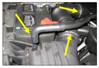
1. Disconnect the negative battery cable. Disconnect the breather hose from the factory air box lid. Loosen the two hose clamps on each end of the factory intake tube.
