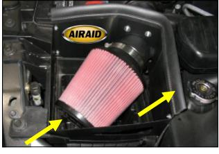
**16.** Install the Airaid Premium Filter on the end of the air filter adapter. Install the supplied weather strip on the Quick Fit panel. Apply the Airaid Foil Decal onto the Panel as shown.
