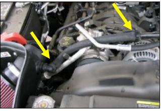
11. Using the supplied pre-formed 3/4" breather hose, connect the nylon fitting to the remaining plastic factory hose as shown. Fasten both ends of the hose using the supplied nylon speed clamps. Adjust the fitting downward to clear the factory intake tube assembly.
