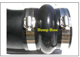
**13.** Slide the hump hose on to the straight end of Airaid intake tube with two #60 hose clamps. (*Note: Leave hose clamps loose until final assembly*).
