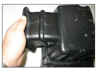
**4.** Using a flat blade screwdriver, carefully unsnap the box inlet from the base and remove it. Reinstall the factory base in the engine compartment with out the inlet.
