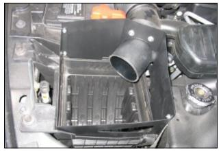
**10.** Install the Airaid Quick Fit assembly on top of the factory air filter base. Relatch the clips, and tighten the hose clamp.
