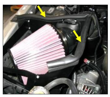
**8.** Mount Airaid Premium Filter to the filter adapter and tighten hose clamp, in addition; press the weather strip onto the top of the Airaid cool air dam. (*Hint: start the install at the top corner of the cold air dam & work toward the edges*)
