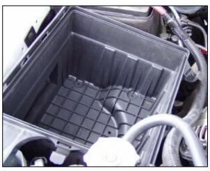
**2.** Unclip the factory air box lid and remove the lid assembly from vehicle.
