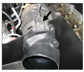
**7.** Re-connect the wire harness to the sensor on top of the Airaid adapter.
