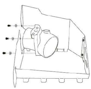
**4.** Assemble the air filter adapter to the cool air dam using the (3) ½-20 bolts and washers provided.
