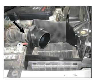
6. <u>Install Airaid intake assembly</u> in place of the factory air box lid & tighten factory hose clamp on intake tube to Airaid system & secure air intake tube to adapter using the factory hose clamp.
