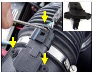
1. Disconnect the negative battery cable and disconnect the electrical connector. Using the T-20 bit loosen the two star head bolts and remove the electrical sensor. (Retain sensor for installation of Airaid Intake System)
