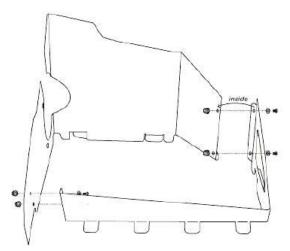
**3.** Assemble Airaid Quick Fit Cool Air Dam panels using the (4) 6/32 screws, washers and nuts provided.
