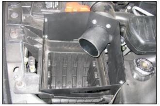
**6.** Install the Airaid Cool Air Dam assembly on top of the factory air filter base. Reconnect the factory intake tube, and tighten the hose clamp.
