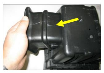
**3.** Using a 13mm socket, remove the air box base from the engine compartment. Using a flat blade screwdriver, carefully unsnap the box inlet from the base and remove it. Reinstall the factory base in the engine compartment without the inlet.
