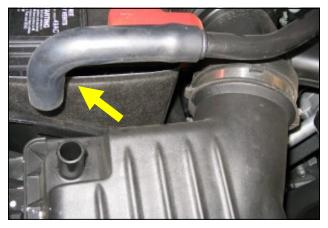
**1.Disconnect The Negative Battery Terminal!** Disconnect the factory breather hose and remove from the vehicle. (Note: 4.7L engines require the removal of the breather hose end section only. 5.7L Hemi required removal of entire hose assembly.
