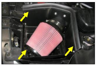
**9.** Install the Airaid Premium Filter on the end of the air filter adapter, and tighten the hose clamp. Install the supplied weather strip on the Cool Air Dam. (Note: start from one end and work your way around to insure proper alignment of weather strip.)
