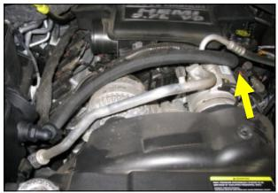
**8. 5.7 Hemi engines only**. Using the supplied straight ¾" hose, connect both ends to the nylon fitting and oil fill nipple as shown. Fasten both ends using the supplied nylon speed clamps. Adjust the nylon fitting downward to clear the factory intake tube assembly.
