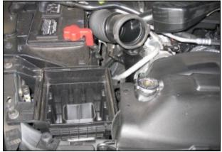
**2.** Loosen the hose clamp on the air box lid and remove the lid from the air box base.
