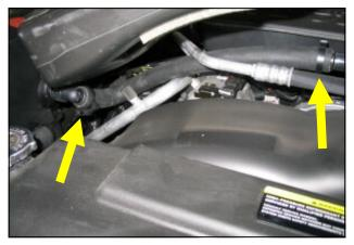
**7. 4.7L engines only**. Using the supplied preformed 3/4" hose, connect the nylon fitting to the remaining plastic factory hose as shown. Fasten both ends of the hose using the supplied nylon speed clamps. Adjust the fitting downward to clear the factory intake tube assembly.
