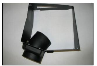
**4.** Using the supplied #6 screws, nuts and washers, assemble the two panels as shown above. Next, install the supplied air filter adapter using the supplied \(^{1}\sqrt{4}\-20\) bolts and washers.
