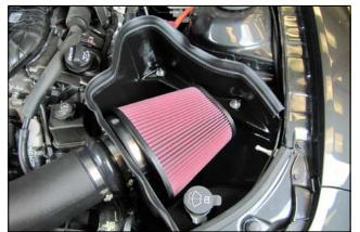
**17.** Install the Weatherstrip onto the Cool Air Box as shown, with the contour rolling away from the Filter. Reinstall the engine cover and oil fill cap.
