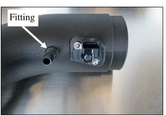
**14.** Install the 1/4" Barbed Fitting into the Airaid Intake Tube as shown. Transfer the Mass Air Flow meter from the factory air box, into the Airaid Tube and secure it using the two 8-32 x 1/2 Screws (#23). Do Not Use The Factory Hardware.
