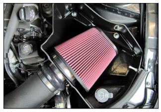
**16.** Install the Airaid Premium Filter onto the Filter Adapter and tighten the clamp.
