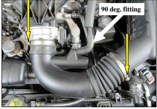
**2.** Disconnect the PCV breather at the 90 degree. fitting. Loosen the two intake tube clamps and remove the tube from the vehicle.
