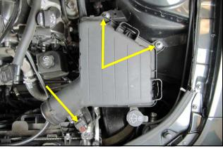
**3.** Disconnect the Mass Air Flow sensor. Using a deep 10mm socket, remove and save the two nuts that secure the factory airbox to the inner fender. These will be reused in step **10**. Lift up and remove the entire airbox and scoop assembly.
