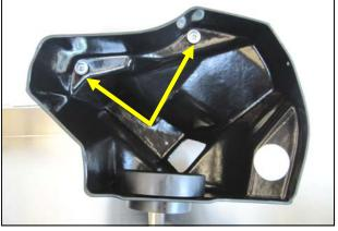
**5.** Transfer the two air box mounting grommets and steel sleeves from the factory air box into the Airaid Cool Air Box.
