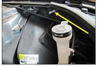
**8.** Remove and save the ground lug from the driver's side inner fender. It will be reused in step #11.
