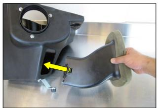
7. Transfer the factory air scoop into the Airaid Cool Air Box. When properly installed, the small locking tab will be inside the Box and the large one will be on the out-
