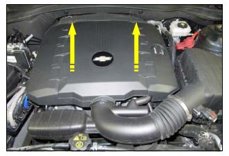
**Disconnect The Negative Battery Terminal.** Remove the oil fill cap and then lift up on the front of the engine cover to remove it from the vehicle. Replace the oil cap to make sure nothing falls into the motor during the install.
