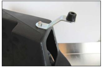
**6.** Turn the Box upside down and mount the Lower Bracket (#10) using the 1/4-20 x 3/4" Hex Bolt (#16), 1/4" Flat Washer (#18), and 1/4" Nylon Lock Nut (#20) as shown. Attach the Plastic Bumper (#11) to the Bracket using the 8-32 x 5/8" Button Head Screw (#24), and the #8 Kep Nut (#25).
