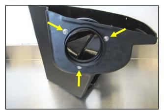
**4.** Install the Filter Adapter onto the Airaid Cool Air Box as shown using three 1/4-20 Button Head Screws (#17), and 1/4" Flat Washers (#18). Refer to the line drawing above for details.
