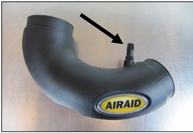
10. Install the Barbed Fitting into the Airaid Intake tube. Apply the Airaid Bubble Decal onto the Intake Tube as shown.
