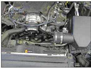
12. Install the coupling hoses onto the air filter housing and throttle body as shown.
