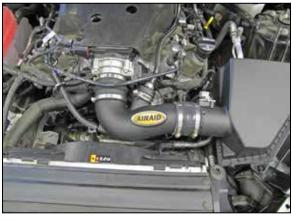
13. Install the intake tube into the coupler at the air filter housing and then into the coupler at the throttle body, adjust the tube for best fit and then secure with the provided hose clamps. Connect the EVAP and crank case vent lines.
