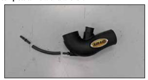
11. Install the provided vent hose and quick disconnect fitting onto the intake tube.
