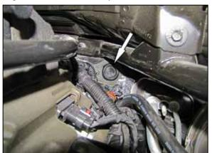
8. Install the provided plug into the hole for the sound tube in the firewall.
