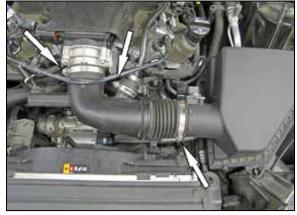
4. Loosen the hose clamp that secures the crank case vent line to the intake tube. Loosen the two hose clamps that secure the intake tube to the air filter housing and throttle body. Disconnect the tube from the air filter housing and throttle body.
