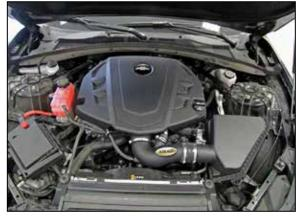
**16. Double check your work!**Make sure there is no foreign material in the intake path. Make sure all clamps, hoses, bolts, and screws are tight. Double check the hood clearance!
