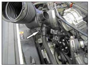
5. Lift up the intake tube to access the sound tube connection and then disconnect the sound tube from the intake tube and remove the intake tube from the vehicle.
