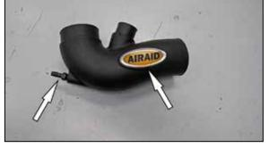
10. Install the AIRAID decal onto the intake tube. Install the provided  $1/4{\rm npt}$  into the intake tube.
