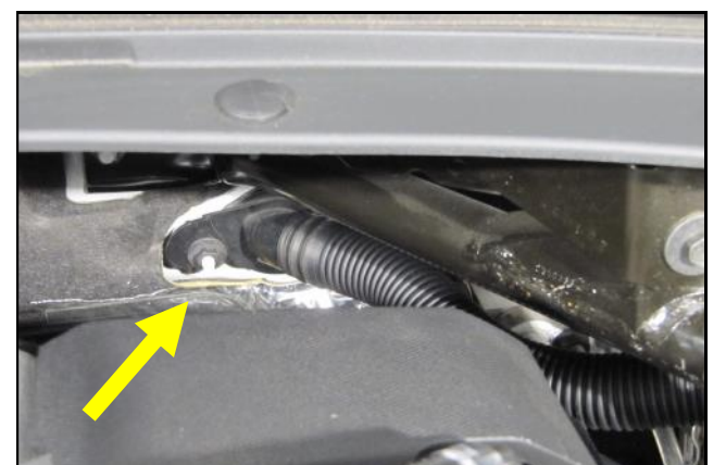
6. At the firewall, remove the 6mm flange nut at the resonator tube base. Turn the tube 1/4 turn Clockwise and remove the entire resonator from the vehicle. It will not be reused.
