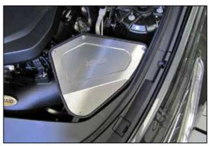
13. Install the provided gasket onto the air box lid, then install the lid onto the air box and secure with the provided hardware.
