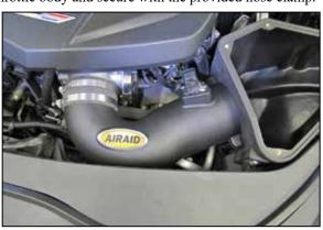
9. Install the intake tube into the air filter housing and then into the coupler on the throttle body, secure the tube to the filter housing using the provided hardware and then secure the tube to the coupler with the provided hose clamp.
