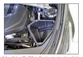
5. Install the AIRAID® air filter housing into the vehicle so the mounting studs engage the factory mounting grommets.
