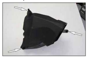
4. Install the provided mounting bracket through the cutout line in the AIRAID® air box and then secure with the provided hardware. Install the provided mounting studs onto the bracket and onto the air filter housing as shown.
