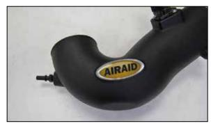
7. Install the provided quick disconnect fitting into the AIRAID® intake tube and then apply the provided decal onto the intake tube.
