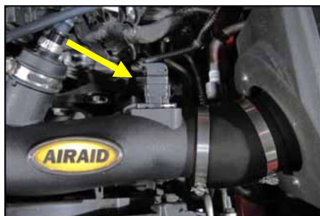
23. Reconnect the Mass Airflow sensor.
