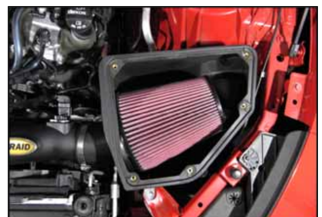
24. Install the Air Filter onto the filter adapter, inside the Airbox.
