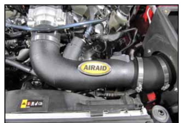
21. Insert the Intake Tube into the Elbow first, then into the Coupler. Tighten all four Clamps.
