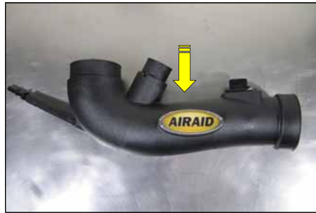
17. Prepare the Intake Tube for Badge installation by cleaning the mounting surface using a Prep Solvent or equivalent. Place the Airaid Badge onto the Intake tube as shown.
