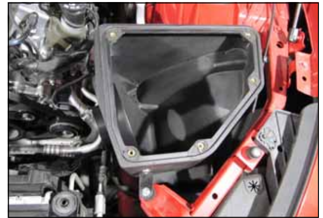
18. Place the Airaid Airbox assembly into the engine compartment as shown, with the mounting posts only fully seated in all three grommets.
