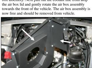
**6.** Install the Adapter Panel (#5) to the MAF Panel (#3) as shown using four 6-32 screws (#12), 6-32 Kep nuts, and #6 flat washers (#14). Attach the Rear Panel (#4) to the MAF Panel using two 6-32 screws.
