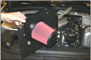
**11. A)** Install the Bracket (#25) on to the Rear Panel (#4) as shown using one 1/4-20 Button Head Screw (#15), 1/4" Flat Washer (#16), and 1/4" Serrated Nut (#17).**B)** Complete the assembly by attaching the Airaid Premium Filter (#1) to the Mass Air Flow Sensor
