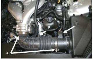
2. A) Loosen the hose clamps on the factory intake
