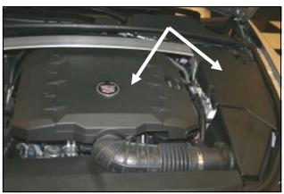
1. Disconnect the negative battery cable. Remove the engine and shock tower covers, if so equipped, by simply pulling up on them, and sliding out from the vehicle. These will be reused later in step 16
