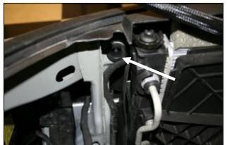
**4.** Use caution not to loose the factory core support grommet while removing the air box assembly. It will be needed in step 13.
