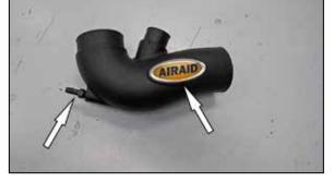
10. <u>Install the AIRAID decal onto the intake tube</u>. Install the provided 1/4npt into the intake tube.
