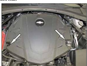
2. Remove the oil cap and bolt that secure the engine cover and then remove the engine cover from the vehicle.
