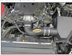
13. <u>Install the intake tube into the coupler at the air filter</u> housing and then into the coupler at the throttle body, adjust the tube for best fit and then secure with the provided hose clamps. Connect the EVAP and crank case vent lines.
