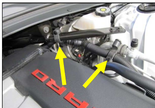
5. Separate the resonator tube from the airbox lid. Follow the tube up to the master cylinder area and disconnect the tube retainers on the strut tower brace and the A/C line.
