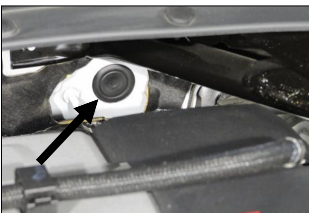
7. Insert the Firewall Plug into the resonator tube hole.
