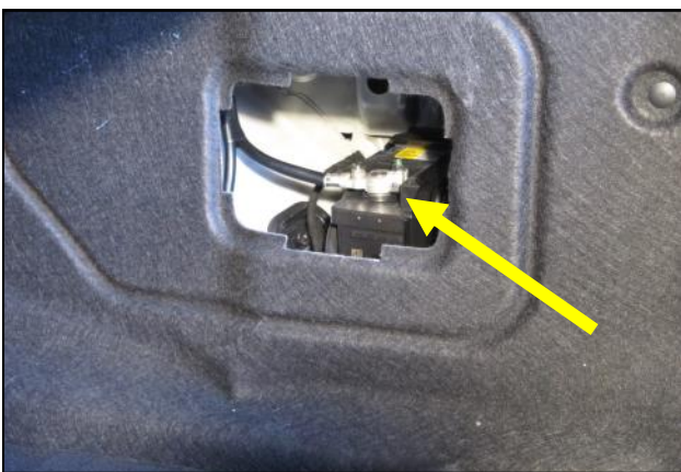
1. Inside the trunk, on the passenger side, locate and remove the battery access panel. Disconnect the Negative battery terminal.
