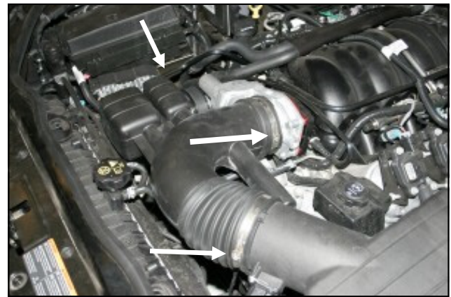
6. Reinstall the intake tube, tighten the two hose clamps, and reconnect the crankcase breather tube. Reinstall the beauty cover, and oil cap in the reverse order that they were removed. Re-connect the negative battery cable!
