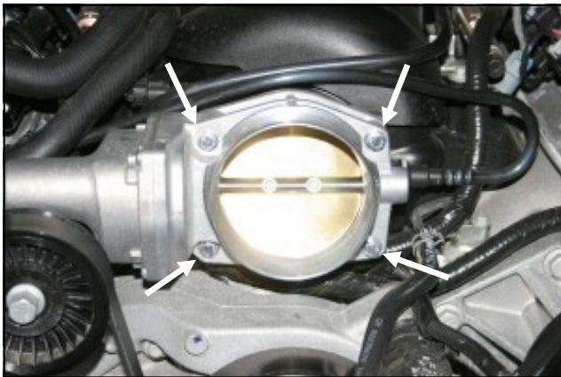
5. Install the provided bolts and washers thru the throttlebody, gasket, and Poweraid Spacer and tighten to the manufacturer's specifications.
