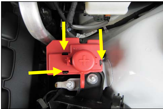
1. Disconnect the negative battery terminal. Depress the three locking tabs on the positive terminal cover and remove it.
