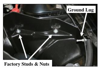
13. Install the Airaid CAB assembly into the vehicle locating the factory grommets over the factory studs. Reinstall the factory nuts from step #3 onto the studs. Reinstall the factory ground lug thru the CAB and thru the side bracket using one flat washer (#17), and one 6mm flange nut (#22). Refer to the line drawing on the first page for reference.
