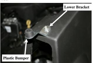
**9.** Turn the CAB upside down and mount the lower bracket (#15) to the bottom of the CAB using one 1/4-20x3/4" hex bolt (#10), 1/4" flat washer (#11), and 1/4" Nylock nut (#25) as shown. Next using one 8-32x5/8" button head screw (#21), and one #8 Kep nut (#26), attach the plastic bumper (#16) to the bracket as shown.
