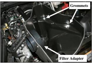
**8.** Reinstall the two steel sleeves and grommets into the Airaid Cold Air Box (CAB) (#3). Next install the filter adapter (#4) into the CAB as shown using three 1/4-20 button head bolts (#19), and 1/4" flat washers (#17). Refer to the line drawing above for details.
