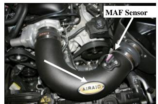
**15.** Install the Airaid Intake Tube (#2) into the hump hose first, and then into the reducing coupler. Adjust for fit, and tighten all four hose clamps. Next install the MAF sensor into the tube and secure it using two 8-32 x 3/8" button head screws (#20). Apply the Airaid Decal onto the Intake Tube a shown.
