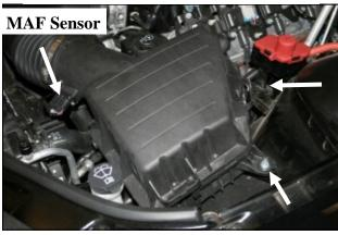
3. Using a deep 10mm socket, remove and save the two nuts that secure the factory airbox to the fender well. Using a 9/32" wrench or a #20 Torx bit, remove the two screws that secure the Mass Air Flow (MAF) sensor into the air intake tube. Without disconnecting the MAF, carefully remove it from the tube and set it out of the way on top of the engine.
