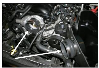
**14.** Install the hump hose (#5) onto the filter adapter using two #64 hose clamps (#9). Next install the reducing coupler (#6) with one #60 hose clamp (#11) on the throttlebody and one #68 hose clamp (#10) on the large and
