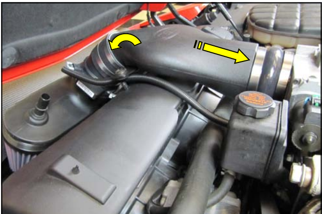
12. Install the Airaid Tube assembly onto the throttle body and lower it downward towards the Mass Air Flow meter. Reconnect the MAF at this time.
