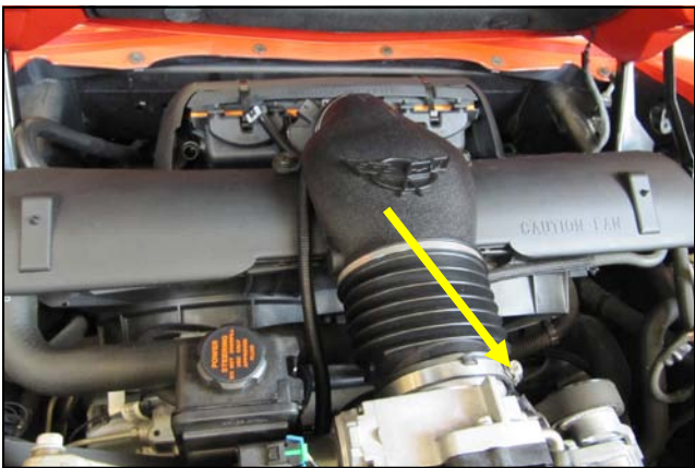
3. Loosen the intake tube clamp on the throttle body.
