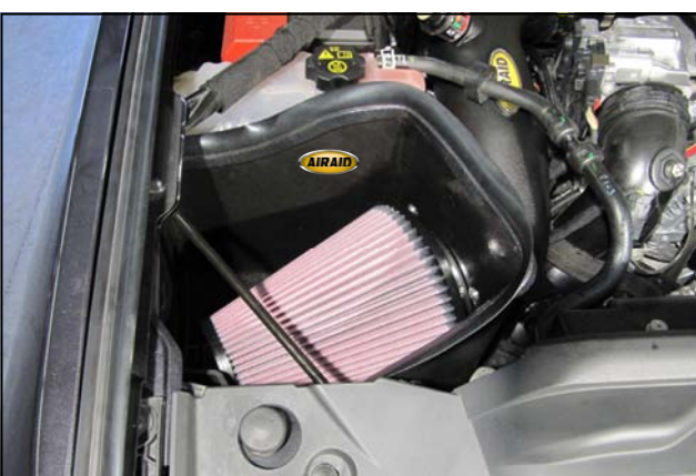
17. Install the Airaid Premium Filter onto the Intake Tube inside of the Cold Air Box. Install the Weather Strip onto the top edge of the Cold Air Box with the contour rolling away from the filter. Reinstall the fender trim and brace.
