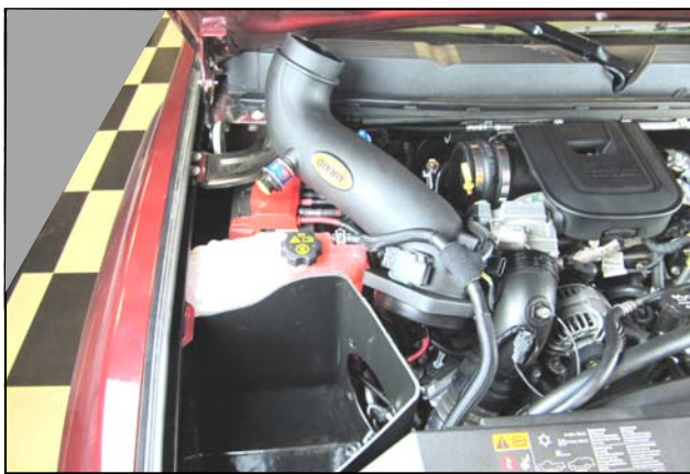
11. Set the Airaid Cold Air Box in the inner fender area as shown.
