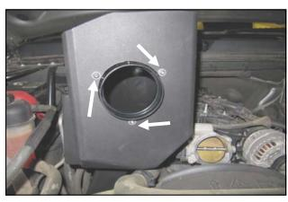
**8.** Install the Filter Adapter (#4) onto the Cold Air Box or CAB (#3) as shown using the three 1/4-20 Button Head Screws (#9) and 1/4" Flat Washers (#10).
