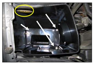
**9.** Install the **CAB** into the engine compartment and secure using three of the tray bolts from step **6.**Apply the Airaid decal inside the Airbox as shown.
