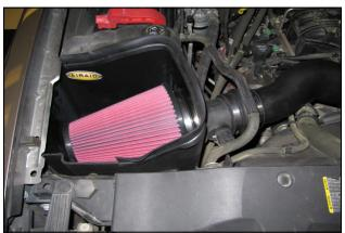
**14.** Install the Airaid Premium Filter (#1) onto the Filter Adapter, and tighten the hose clamp. Install the weather strip (#8) onto the Airaid Cold Air Box. (*Hint: Start from one corner and work your way around for ease of install.*)
