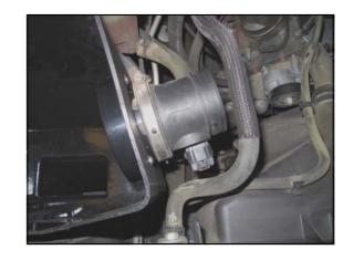
**10.** Transfer the Mass Air Flow sensor from the factory airbox onto the Filter adapter. Reconnect the MAF.
