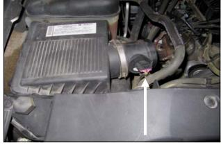
**5.** Disconnect the **MAF** sensor and remove the factory airbox and sensor from the vehicle.
