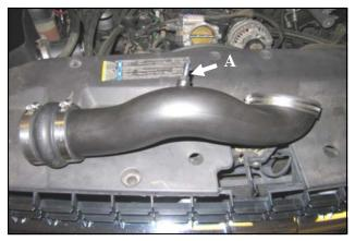
11. **A**) Install the 1/4" NPT Barbed Fitting (#12)into the Airaid Intake Tube(#2).
