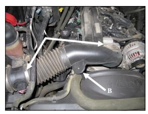
**3.A.**) Loosen the clamps securing the factory intake tube to the throttlebody and the Mass  $\bf A$ ir Flow  $\bf M$ eter, or  $\bf M \bf A \bf F$ .
