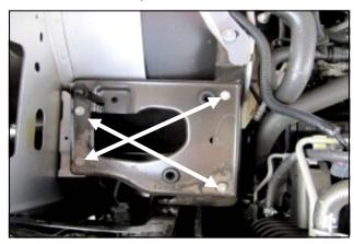
**6.** Remove the four tray bolts and the airbox mounting tray. Three of the bolts will be reused in step **8.**
