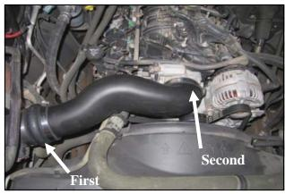
**12.** Install the Airaid Intake Tube assembly onto the **MAF** first, and then onto the throttlebody. Adjust for fit, and tighten all hose clamps. Reinstall the hose anchor into the Airaid Intake Tube.
