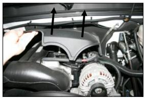
**1.** <u>Disconnect the negative battery cable.</u> Remove the factory beauty cover by lifting up on the front, and then pulling the cover towards the front of the vehicle. It is only held in place by grommets.
