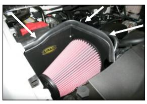
14. Install the Airaid Premium Filter (#1) onto the air filter adapter, and tighten the hose clamp. Next install the provided weather strip (#9) onto the top of the CAD. For ease of install, start at the inner fender, and work your way towards the radiator. Reinstall the beauty cover.
