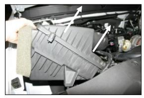
**4.** Loosen two hose clamps on the factory intake tube. One at the throttlebody, and one where it clamps to the factory airbox. Remove the factory intake tube from the vehicle.
