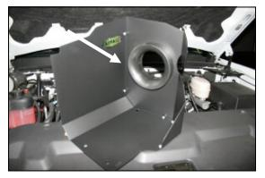
8. Assemble the Cool Air Dam panels (CAD) (#2 & #3) using five 6-32 x 5/16" screws (#10), #6 flat washers (#11), and 6-32 keps nuts (#12). Next install the air filter adapter (#5) into the panels as shown with the hole for the Mass Air Flow sensor facing up, using three  $1/4 - 20 \times 1/2$ " button head bolts (#14), and 1/4" flat washers (#15). Apply the Airaid Foil Decal onto the Panel as shown.
