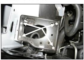
**7.** Using a 10mm socket, remove four bolts, and then remove the factory airbox mounting plate from the vehicle.
