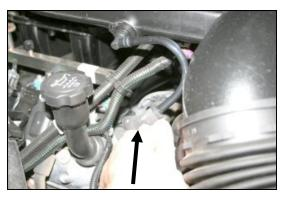
**2.** Disconnect the factory breather hose at the valve cover by pulling the small black tab on the fitting towards the front of the vehicle, and then to the right.
