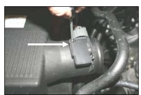
**5.** Remove, and set aside the **MAF** (**M**ass **A**ir **F**low) sensor from the factory airbox. This will require a T15 Torx Bit.
