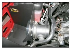
**11.** Reinstall the **MAF** sensor onto the filter adapter, and tighten the clamp.
