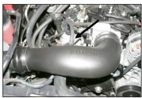
**14.** Install the Airaid Intake Tube into the hump hose first, and then onto the throttle body. Adjust it for fit, and tighten the hose clamps. Next install the 3/8" x 14" breather hose (#8) between the 1/4" NPT x 3/8" barbed fitting in the tube, and the factory port on the valve cover.
