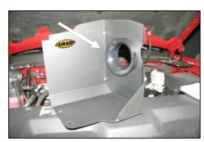
**9.** Assemble the Cool Air Dam panels (CAD) (#2 & #3) using five 6-32 x 5/16" screws (#10), #6 flat washers (#11), and 6-32 keps nuts (#12). Next install the air filter adapter (#5) into the panels as shown using three 1/4 - 20 x 1/2" button head bolts (#13), and 1/4" flat washers (#14). Apply the Airaid Decal as shown.
