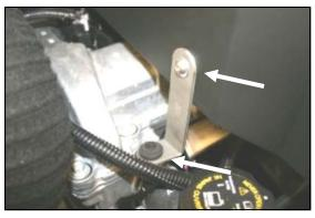
12. Install the small factory grommet removed in step #5 into the supplied bracket (#14). Next slip the installed grommet over the stud on the front of the engine, and bolt the bracket to the CAD using one 1/4-20x 1/2" button head bolt (#7), 1/4" flat washer (#8), and 1/4" serrated nut (#9).
