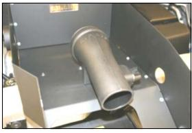
10. Install the Airaid Intake Tube onto the CAD using two 1/4-20 x 1/2" button head bolts (#7) and 1/4" flat washers (#8), threaded up from the bottom of the **CAD**.
