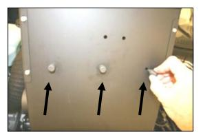
7. Install the three silicone bumpers (#15) into the three holes in the bottom of the Cool Air Dam, as shown.
