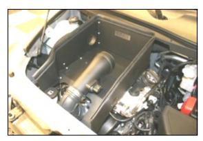
11. Install the assembled CAD into the vehicle by lowering the front into the vehicle first, and then aligning the two grommets on the studs at the rear of the engine. Push down firmly on the rear of the CAD to seat the grommets. Next slide the factory rubber elbow onto the Airaid Intake Tube.
