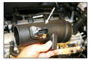
**9.** Install the Mass Air Flow sensor removed in step #4, into the Airaid Intake Tube (#5) using the two 8/32"x 3/8" button head screws (#10). **DO NOT USE THE FACTORY SCREWS!**
