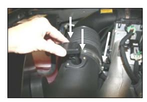
12. Re-position the factory intake tube onto the Airaid tube, and tighten the hose clamp. Next reinstall the Mass Air Flow sensor into the Airaid tube using the two provided Button Head screws (#8). Do not use the factory screws! Do not over tighten!
